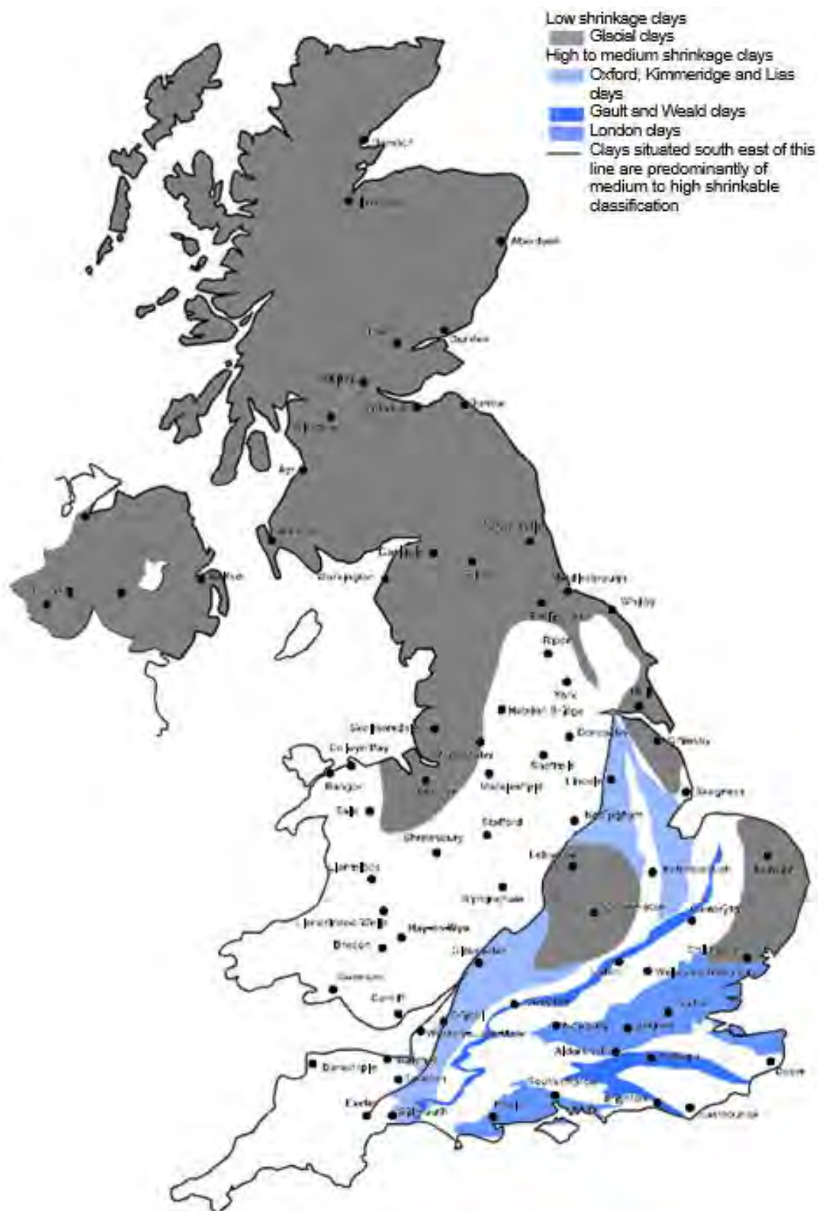
Diagram 1.15 – Guidance on the Location of Highly Shrinkable Clay Soils
