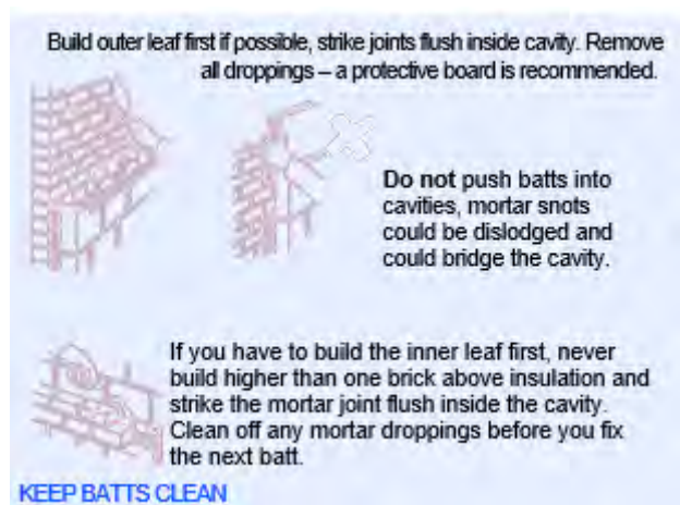
Diagram 2.74: Installation of full fill insulation batts – keep batts clean
