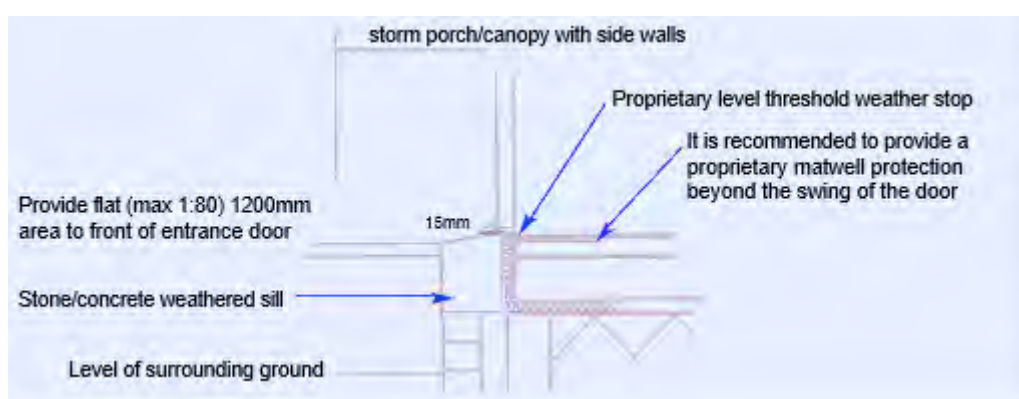
Diagram 2.82: Level threshold with porch/canopy protection
