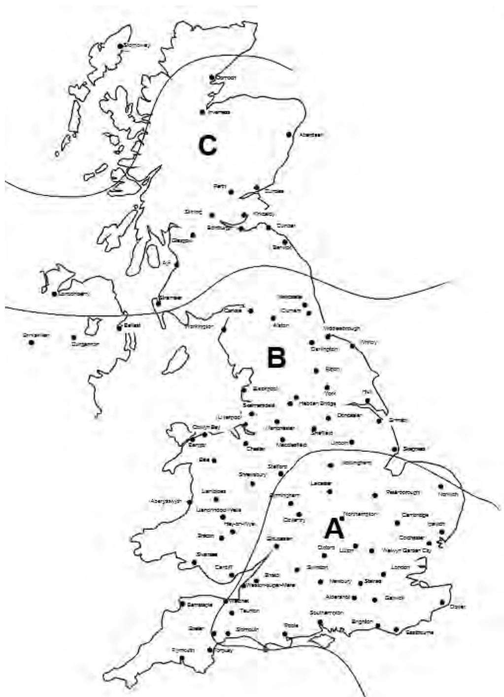
Diagram 2.174: Wind zones – British Isles. Parts of Scotland are outside Zone C and as such, roofs in this
