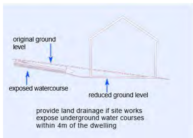
Diagram 1.26: Ground Water Exposed by Site
